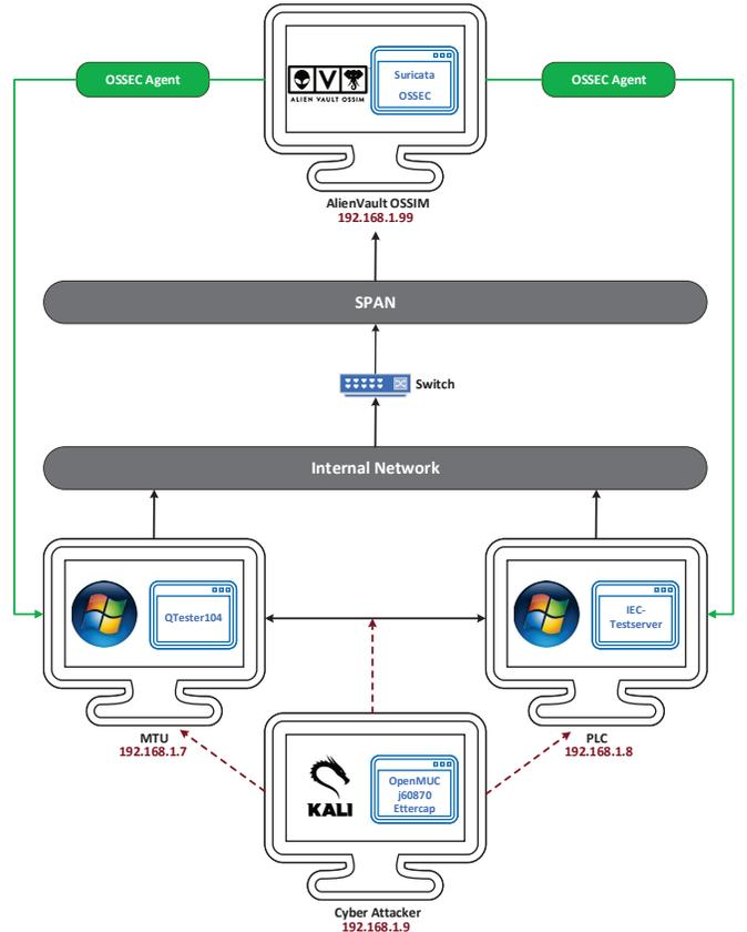
Fig. 2. Testbed for emulating cyber attacks against IEC-104.
