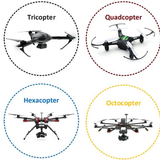
Figure 3: Rotary-wing UAVs.
