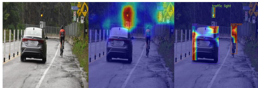
Figure 2. An illustration showcasing an original input image processed by the XAI component, alongside the output heatmap highlighting significant areas within the entire image, as well as individual heatmaps highlighting detected objects within the scene.
